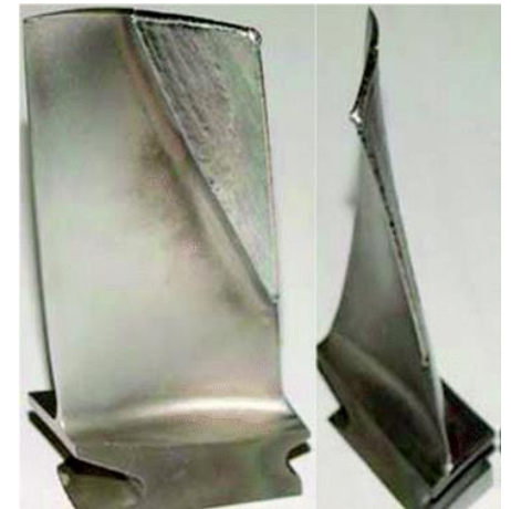
Blisk airfoil repaired by laser DED
