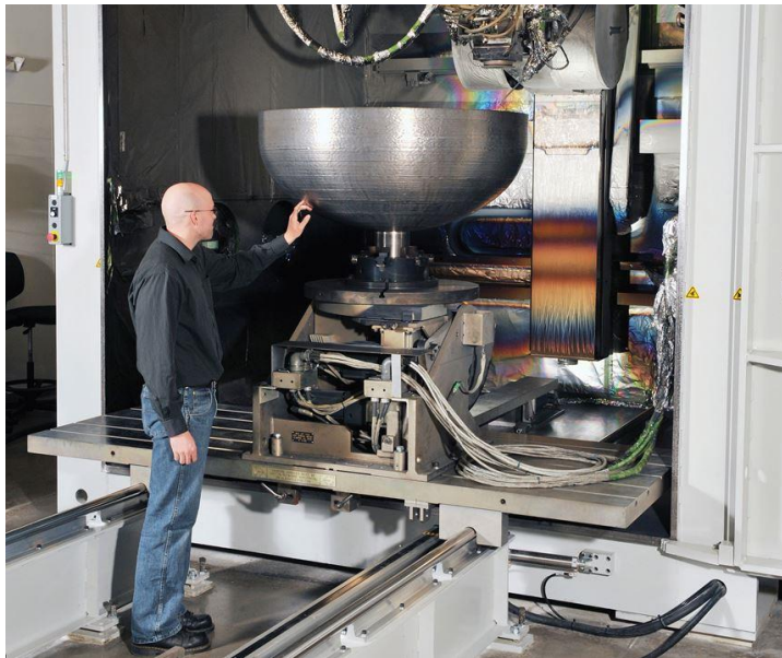
Manufacturing of a Lockheed Martin titanium satellite propellant tank using EBAM.
